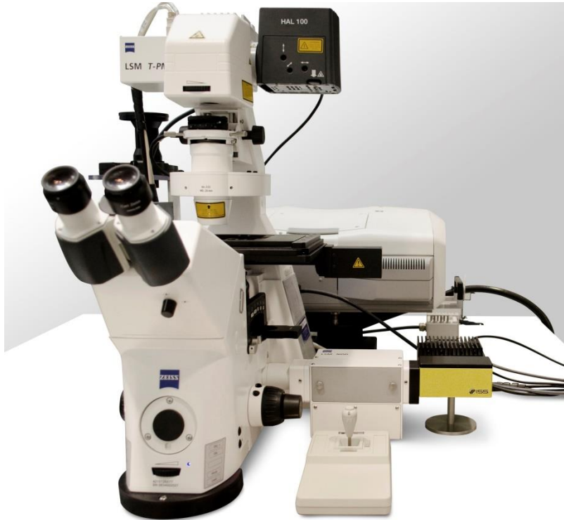
Figure 1.1 Model LSM780 confocal microscope. The ISS detector (featured on the right section / yellow color) is added to the NDD port
