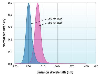
Figure 1. Normalized spectra of the 280-nm and 300-nm LEDs. FWHM is about 12-nm for each LED. The LEDs do now show any additional extraneous emission up to 750-nm: is not detectable in this wavelength range.
