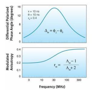
Figure 3. Calculated differential phase and modulated anisotropy curves for  $\tau = 10$  ns,  $\theta = 10$  ns and r $_0 = 0.4$  [2]
