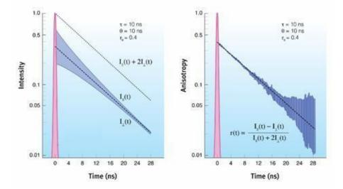
Figure 1. Time-dependent anisotropy decays (left) and calculated anisotropy decay (right). [2]
