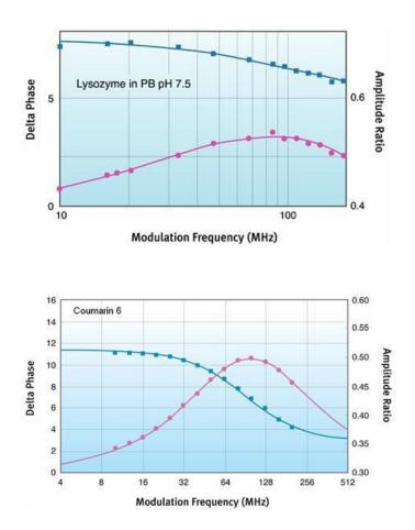
**Figure 4**. Frequency-domain anisotropy decays (Differential Polarized Phase Angle and Amplitude Ratio) of Lysozyme in phosphate buffer pH 7.5 measured with a 300-nm LED. The emission was collected using a WG320. Calculated values for  $\theta_1 = 0.8$  and  $\theta_2 = 6.08$ , R0 = 0.17 with  $\tau_1 = 0.7$  ns and  $\tau_2 = 2.58$  ns, f1 = 0.26.
